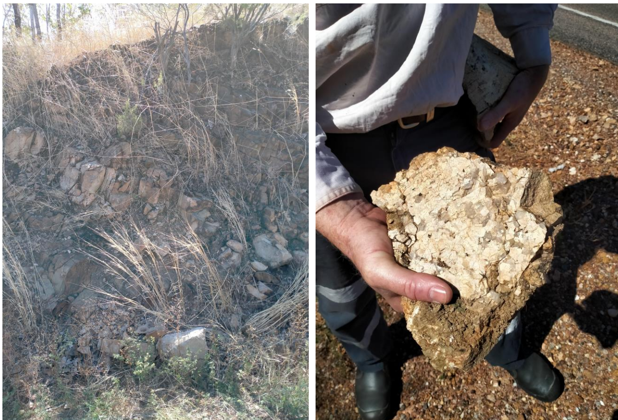
Figure 3.9 Mapped weathered pegmatite at a Stuart Highway road cutting
